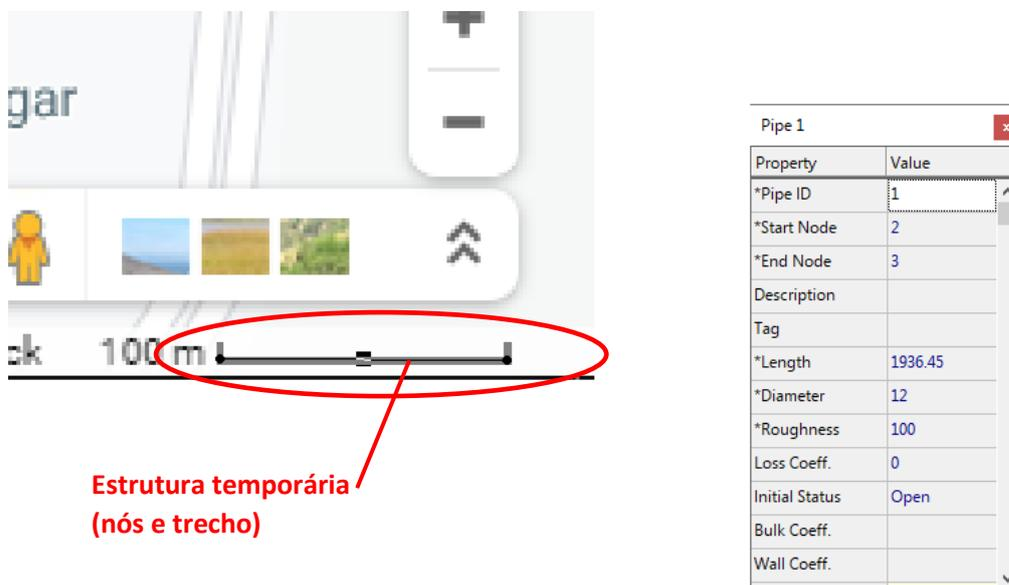
The image shows a screenshot of the EPANET software interface. On the left, a map displays a temporary pipe structure (a line segment between two nodes) highlighted with a red oval. A red arrow points from this oval to a red text label: "Estrutura temporária (nós e trecho)". On the right, a window titled "Pipe 1" displays the properties of the selected pipe segment.
